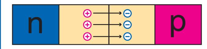
The depletion zone prevents any significant electric current flow if an external voltage is placed across the diode with the same polarity as the built-in potential; this is the reverse bias phenomenon.
