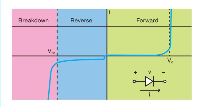
If the reverse bias is beyond the peak inverse voltage (PIV), reverse breakdown occurs. This causes a large increase in current that usually damages the device permanently, an effect used deliberately in the avalanche diode.
